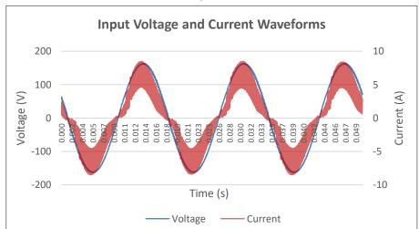
Input AC Current Waveform (ITHD = 15.18%, 50% Load)
